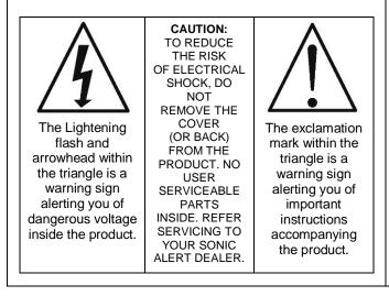
WARNING: TO PREVENT FIRE OR SHOCK HAZARD, DO NOT EXPOSE THIS APPLIANCE TO RAIN OR MOISTURE.
