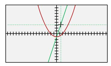
**Note:** In the picture above the cursor is shown using green lines. This indicates that f(x) mode is currently set for f2(x). All the graph attributes (scale settings, solving for zeros, cursor settings, etc.), are set for f2(x). To switch back to f1(x) return to f(x) mode and select softkey **f1**<>**f2**.
