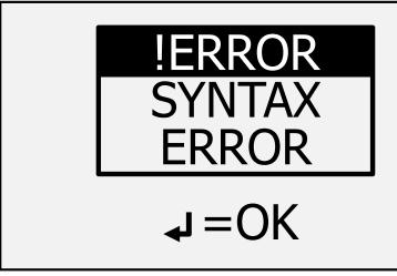
Sometimes you'll enter things incorrectly, such as not closing a bracket or dividing by zero. In this case, you'll get a **SYNTAX ERROR** message like the image at left.
