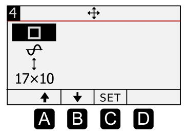
The fourth screen is the RANGE screen, indicated by  $\clubsuit$ . Here you can automatically set the size of the x and y axis as appropriate for the equation that is being graphed. The four settings are as follows:
