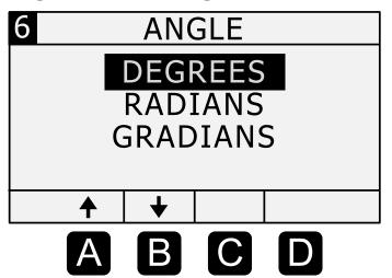
Use the A and B softkeys to select the angle mode.
