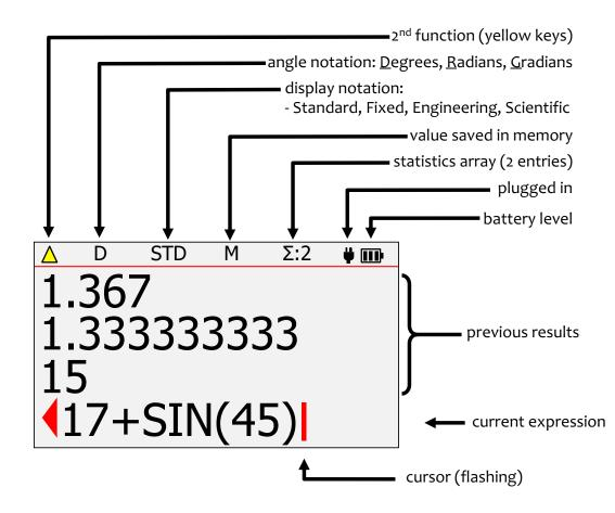
The characters above the horizontal red line at the top of the screen show the **status line** of the calculator. If the battery symbol is animated, this indicates that the battery is being charged. Some of the characters in the status line may not appear at all times. For example, if there is no entry in memory, or if the statistics register is currently empty, these items will not appear.
