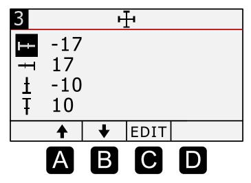
The third screen, indicated by the + symbol, is used to manually adjust the range for the x and y axes. Note that the SciPlus will never allow you to enter a minimum value that is larger than the maximum value for the x or y axis. Use A B to select the axis end point you wish to adjust, and C to edit the value.
