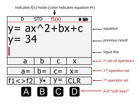
First operator set: Push f(x) once. The four soft keys allow you to use the variables a, b, c, x to define a function in the form y = f(a,b,c,x).
